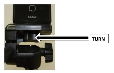
To extend the head of the tripod so it is taller (if needed): Turn knob at the base of the head to the right > Pull to extend > Turn the knob to the left to lock it
