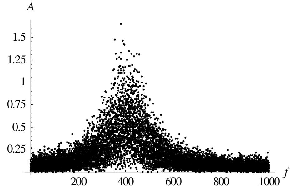
The output signal is not the white noise but a colored noise. It has a maximum at the resonance frequency (here  $f_0=400$  Hz), so that the ear can hear this frequency above the hiss.
