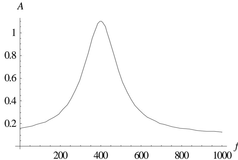
Fourier spectrum of the output (filtered) signal with the white-noise input
