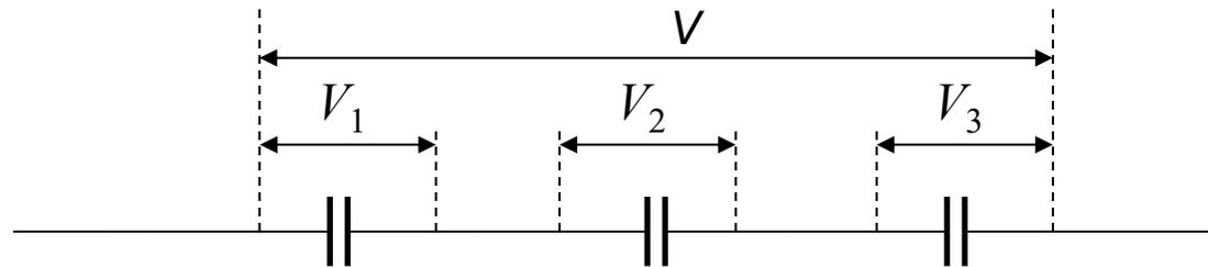
Here voltages add up whereas the charge is common (on each of the capacitors the same)
