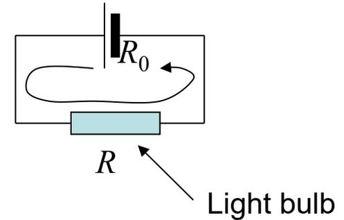
Solution: (a) The total dissipated power in the circuit is equal to the power of the electromotive force:
