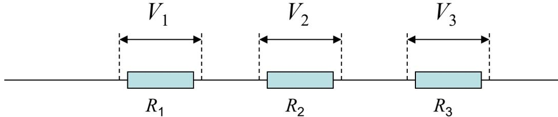
As the current  $I$  through each of serially connected resistors is the same, one can use Ohm's law and write
