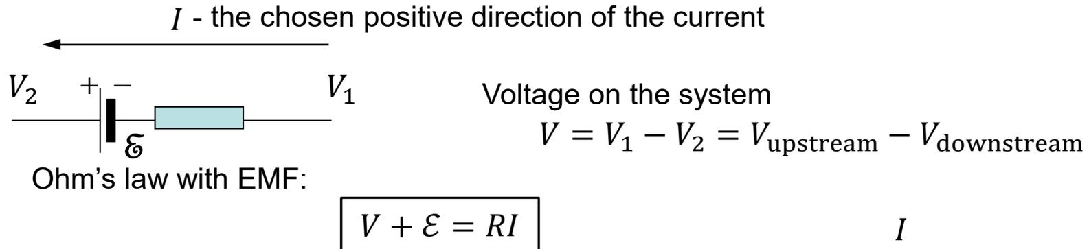
Consider the simplest closed circuit: battery and the load.
