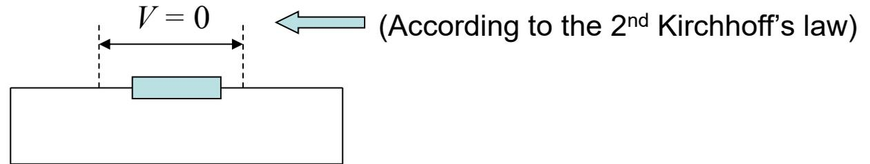
shows that the electric current is zero. Indeed, there is no reason for the current to flow along the closed loops in the circuit because the total change of the potential across any loop is zero. What causes electric charges to flow are non-electric forces such as chemical forces in batteries. These forces are not potential forces because the work done by these forces along closed loops is nonzero. This is exactly the reason for the currents to flow in closed electric circuits.
