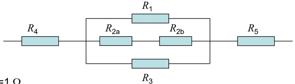
Solution: We at first replace the serially connected resistances  $R_{2a}$  and  $R_{2b}$  by the effective resistance  $R_2 = R_{2a} + R_{2b}$ . Then we replace the central group of parallel connected resistances by the effective resistance
