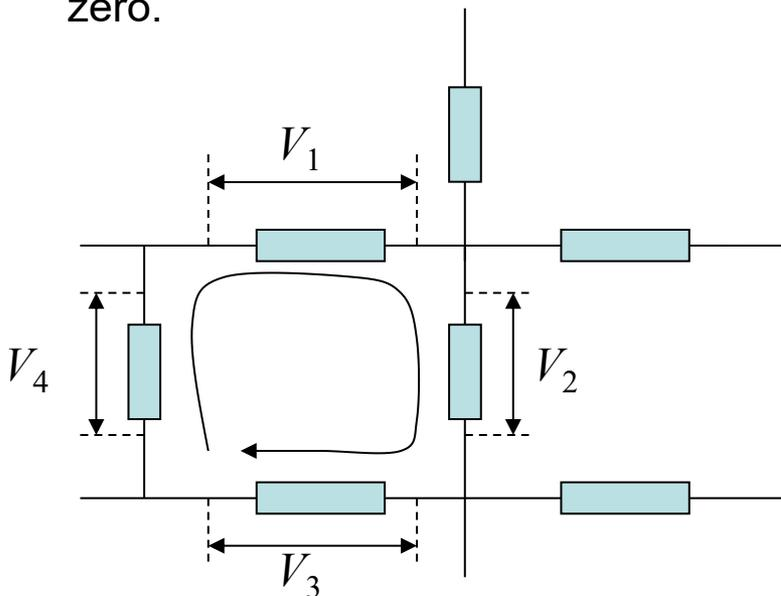
$$V_1 + V_2 + V_3 + V_4 = 0$$
