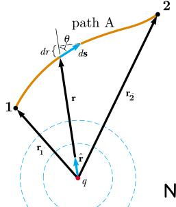
Work done by electric force  $\vec{F}$  as charge moves infinitesimal distance  $d\vec{s}$  along  $\operatorname{Path} A = dW$
