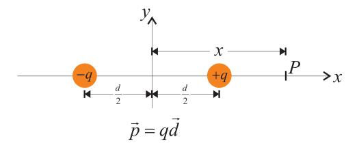
Consider potential of point  $% \left( x\right) =\left( x\right) +\left( x\right) =0$  at distance  $x>\frac{d}{2}$  from dipole P
