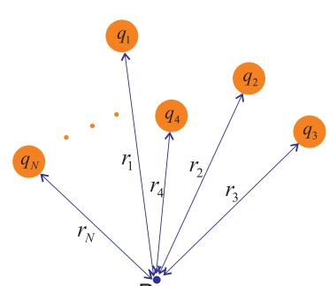
For a total of N point charges potential V at any point P can be derived from **principle of superposition**
