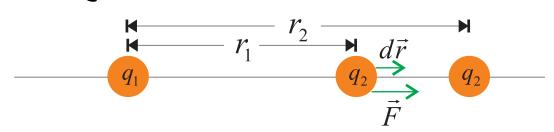
Suppose charge  $q_2$  moves from point 1 to 2
