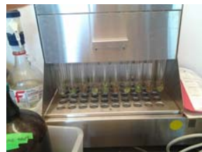
Figure 2: Aim 600 digestion system used for digesting Brassica juncea tissues
