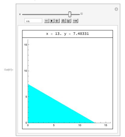
In[78]:= (\*Step 1 (Quantities): x[t]=distance from bottom of ladder to wall, y[t]=height where ladder touches the wall. Both depend on time t.\*) (\*Step 2: What are the relations between these quantities:\*) x[t]^2+y[t]^2 == 15^2
