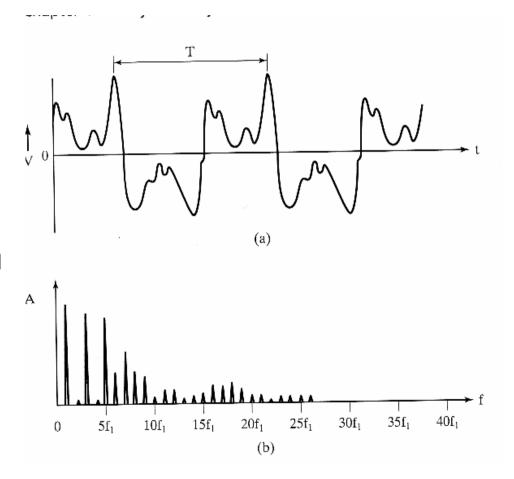
• Fourier spectrum of periodic signals consist of regularly-spaced spikes corresponding to the fundamental and overtones. This is a <u>discrete</u> Fourier spectrum
