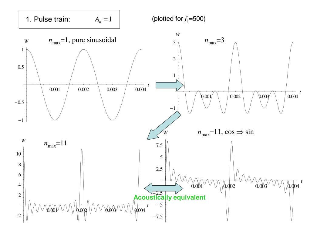
The set of the amplitudes  $A_n$  of a signal (complex wave) is called the <u>Fourier spectrum</u> of the signal. For a periodic signal the Fourier spectrum can be plotted as a series of spikes at the frequencies  $f_n$ with the hights proportional to the corresponding amplitudes  $A_n$ .
