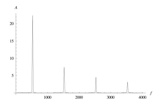
Here is the Fourier spectrum of a square wave. One can see the fundamental frequency  $f_1$ =500 Hz and odd overtones at 1500 Hz, 2500 Hz, 3500 Hz, etc. Even overtones at 1000 Hz, etc. are absent for the square wave.
