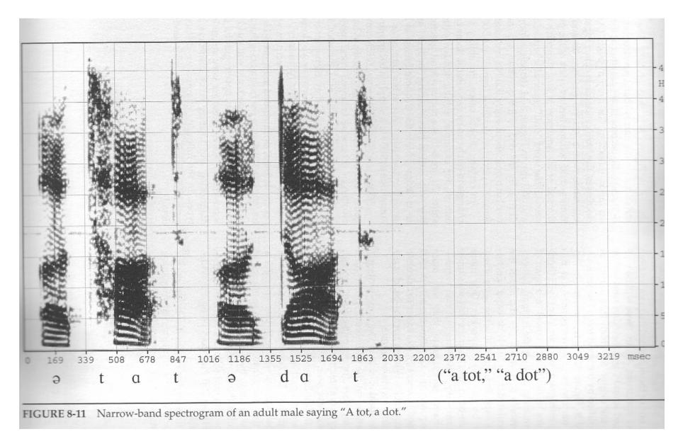
A narrow-band spectrogram: One can see fundamentals and overtones (black stripes) along the vertical direction. The frequency of the fundamental and overtones change with time during the speech. Formants are seen as darker regions.
