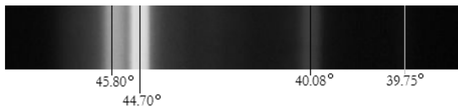
Figure 8.2 A typical diffraction pattern for one fringe from the light emitted by Mercury
