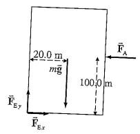
Since this is a negative torque, the building will tend to rotate clockwise, which means it will rotate back down to the ground. Thus the building will not topple.
