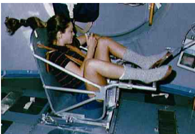
h / Astronaut Tamara Jernigan measures her mass aboard the Space Shuttle. She is strapped into a chair attached to a spring, like the mass in figure g. (NASA)
