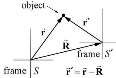
**Figure 11.1** Two reference frames  $S$  and  $S'$ .
