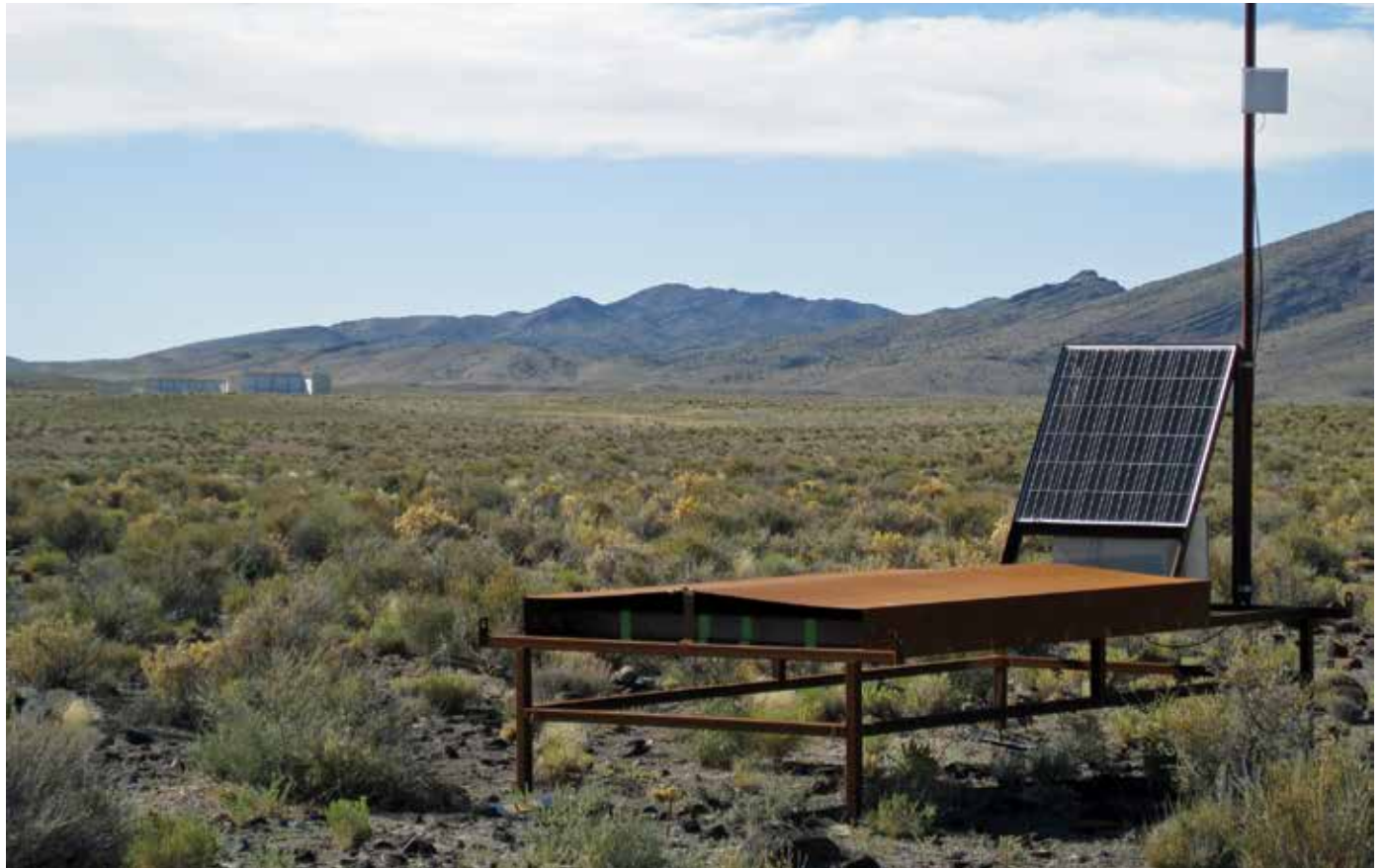
▲ TELESCOPE ARRAY This solar-powered scintillation detector measures the strength and direction of air-shower particles created by incoming cosmic rays. The setup is how it appeared in 2014, when the collaboration announced its hotspot detection.
