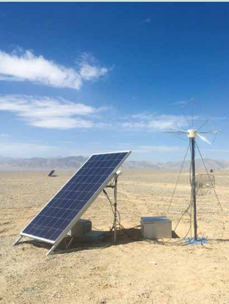
◀ GRAND FUTURE Far left: This windswept site in western China is the home of the growing Giant Radio Array for Neutrino Detection. Standing at the site are Xiang-Ping Wu and Huang Yan (National Astronomical Observatories of China). Near left: The setup for site survey operations. Scientists used easily moved antennas to measure background noise.
