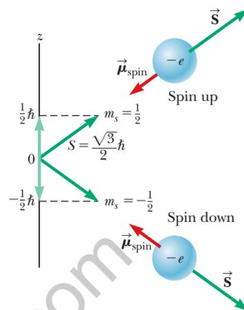
**Figure 42.17** Spin angular momentum  $\vec{S}$  exhibits space quantization. This figure shows the two allowed orientations of the spin angular momentum vector  $\vec{S}$  and the spin magnetic moment  $\vec{\mu}_{\text{spin}}$  for a spin- $\frac{1}{2}$  particle, such as the electron.
