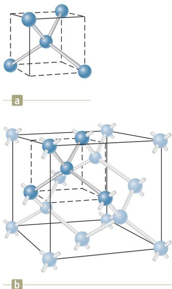
**Figure 43.13** (a) Each carbon atom in a diamond crystal is covalently bonded to four other carbon atoms so that a tetrahedral structure is formed. (b) The crystal structure of diamond, showing the tetrahedral bond arrangement.
