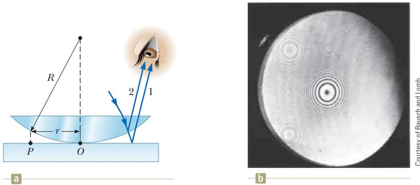
**Figure 37.11** (a) The combination of rays reflected from the flat plate and the curved lens surface gives rise to an interference pattern known as Newton's rings. (b) Photograph of Newton's rings.
