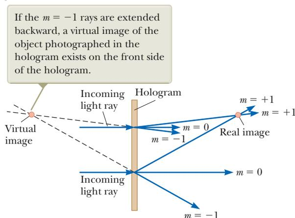
**Figure 38.19** Two light rays strike a hologram at normal incidence. For each ray, outgoing rays corresponding to  $m = 0$  and  $m = \pm 1$  are shown.
