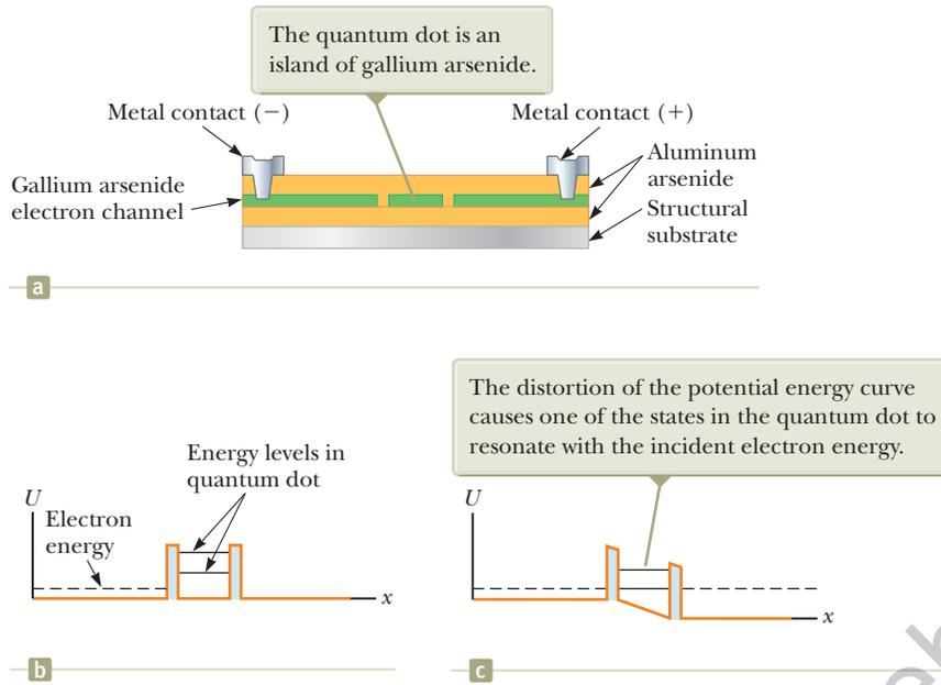
**Figure 41.12** (a) The physical structure of a resonant tunneling device. (b) A potential-energy diagram showing the double barrier representing the walls of the quantum dot. (c) A voltage is applied across the device.
