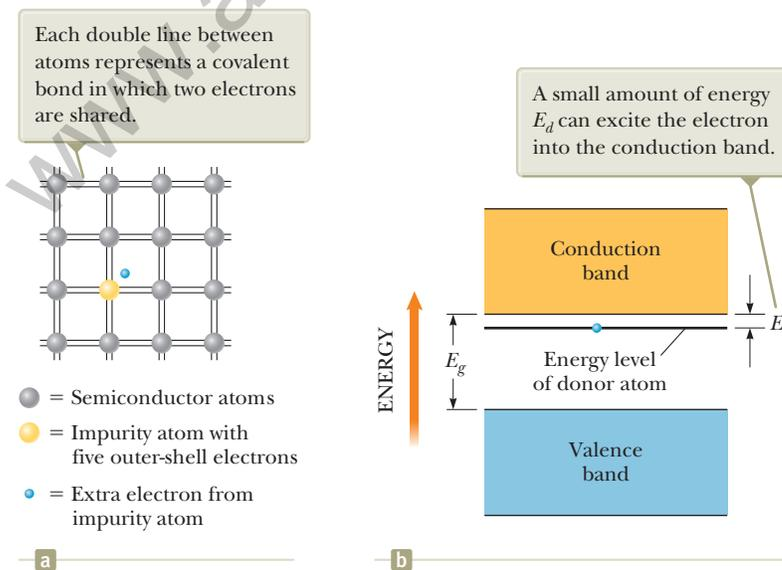
**Figure 43.26** (a) Two-dimensional representation of a semiconductor consisting of Group IV atoms (gray) and an impurity atom (yellow) that has five outer-shell electrons. (b) Energy-band diagram for a semiconductor in which the nearly free electron of the impurity atom lies in the energy gap, immediately below the bottom of the conduction band.
