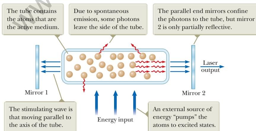
Figure 42.29 Schematic diagram of a laser design.
