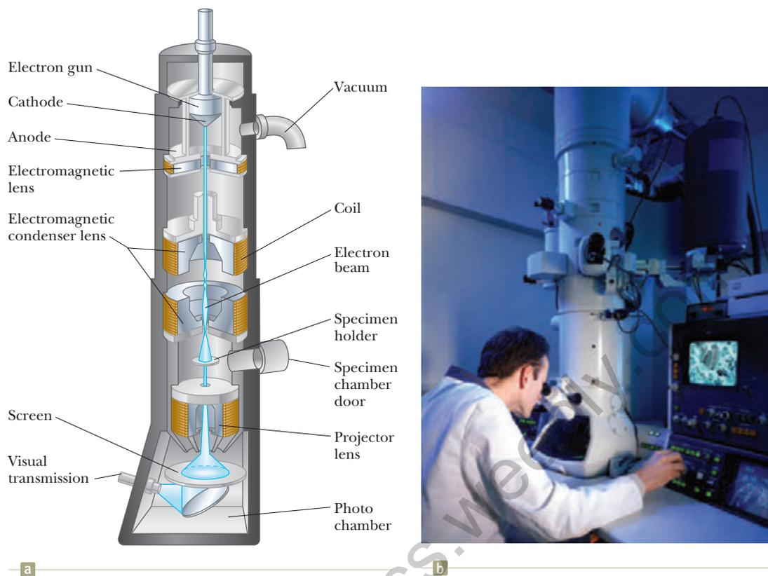
**Figure 40.16** (a) Diagram of a transmission electron microscope for viewing a thinly sectioned sample. The “lenses” that control the electron beam are magnetic deflection coils. (b) An electron microscope in use.
