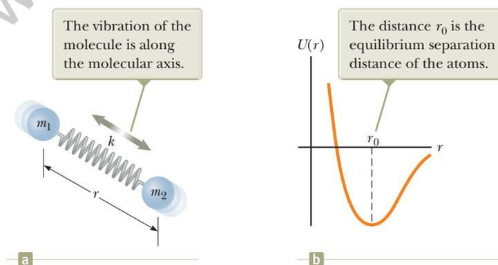
**Figure 43.6** (a) Effective-spring model of a diatomic molecule. (b) Plot of the potential energy of a diatomic molecule versus atomic separation distance. Compare with Figure 15.11a.
