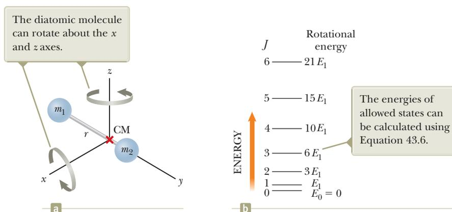
**Figure 43.5** Rotation of a diatomic molecule around its center of mass. (a) A diatomic molecule oriented along the  $y$  axis. (b) Allowed rotational energies of a diatomic molecule expressed as multiples of  $E_1 = \hbar^2/I$ .
