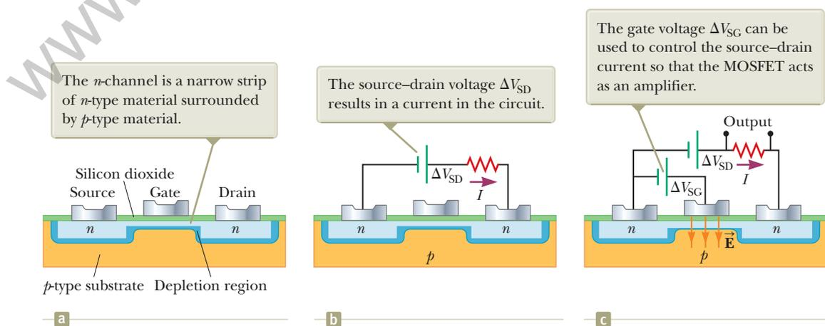
**Figure 43.31** (a) The structure of a metal-oxide-semiconductor field-effect transistor (MOSFET). (b) A source-drain voltage is applied. (c) A gate voltage is applied.
