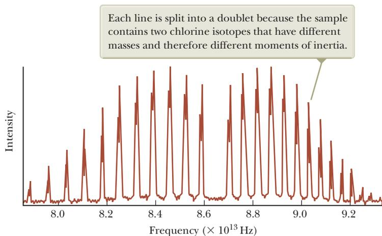
**Figure 43.9** Experimental absorption spectrum of the HCl molecule.
