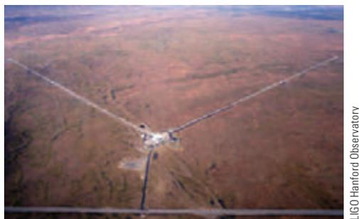
**Figure 37.14** The Laser Interferometer Gravitational-Wave Observatory (LIGO) near Richland, Washington. Notice the two perpendicular arms of the Michelson interferometer.
