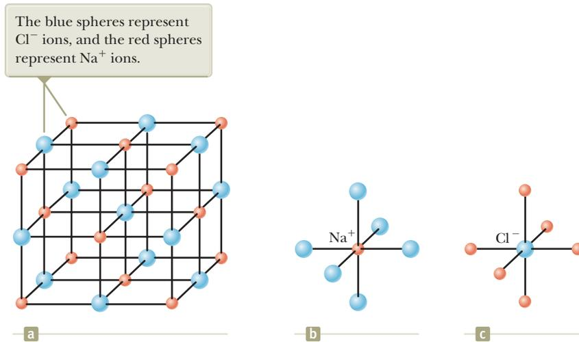
**Figure 43.11** (a) Crystalline structure of NaCl. (b) Each positive sodium ion is surrounded by six negative chlorine ions. (c) Each chlorine ion is surrounded by six sodium ions.
