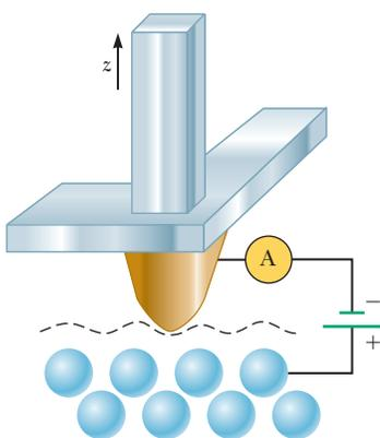
**Figure 41.11** Schematic view of a scanning tunneling microscope. A scan of the tip over the sample can reveal surface contours down to the atomic level. An STM image is composed of a series of scans displaced laterally from one another. (Based on a drawing from P. K. Hansma, V. B. Elings, O. Marti, and C. Bracker, *Science* 242:209, 1988. © 1988 by the AAAS.)
