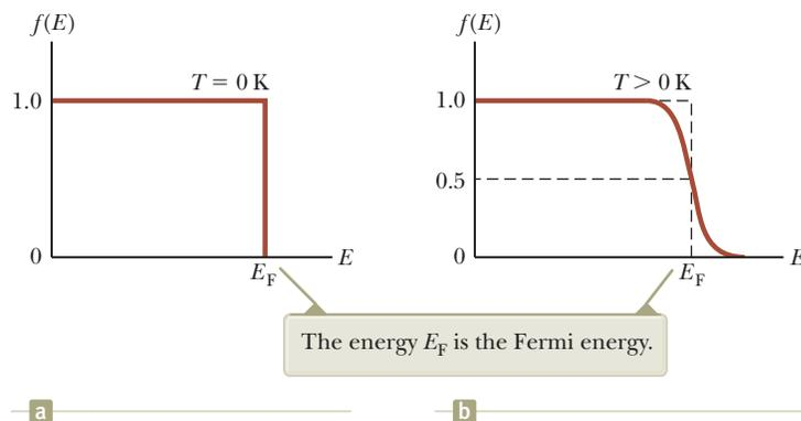
**Figure 43.16** Plot of the Fermi–Dirac distribution function  $f(E)$  versus energy at (a)  $T = 0$  K and (b)  $T > 0$  K.
