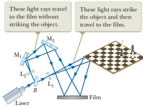
**Figure 38.18** Experimental arrangement for producing a hologram.
