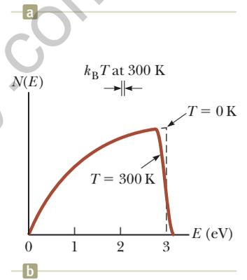
**Figure 43.17** Plot of the electron distribution function versus energy in a metal at (a)  $T = 0$  K and (b)  $T = 300$  K.
