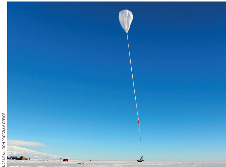
The balloon-mounted ANITA experiment surveys more than a million square kilometres of Antarctic ice for signals from cosmic rays
