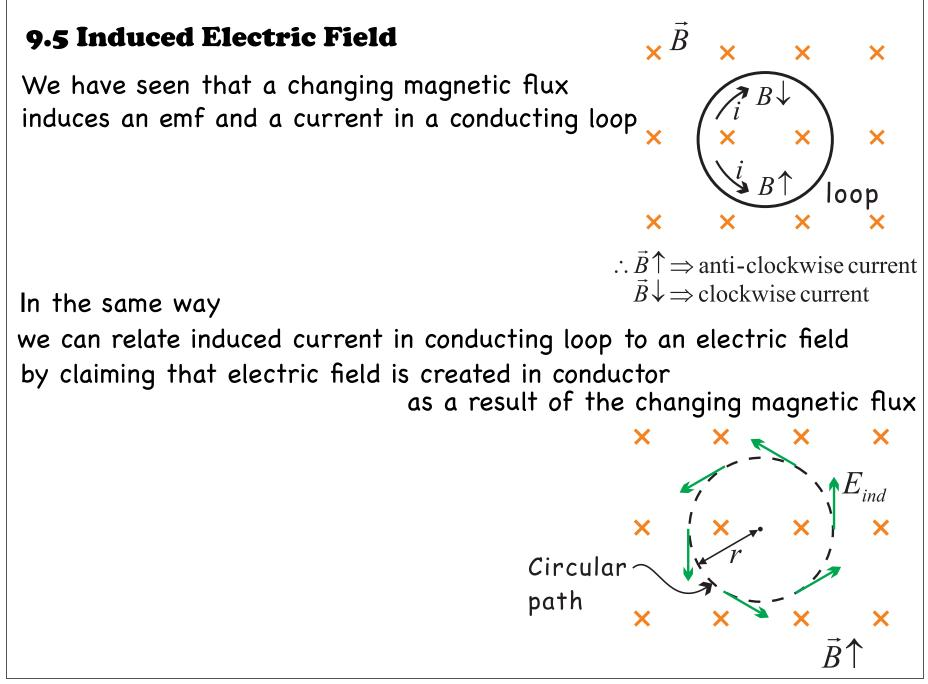
Induced electric field is nonconservative unlike electrostatic field produced by stationary charges We can illustrate this point by considering conducting loop of radius rsituated in uniform magnetic field that is perpendicular to plane of loop
