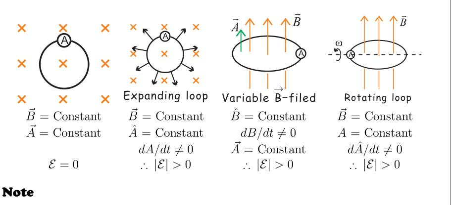
Induced emf drives a current throughout circuit similar to function of a battery Difference here is that induced emf is distributed throughout circuit consequence we cannot define a potential difference between any two points in circuit
