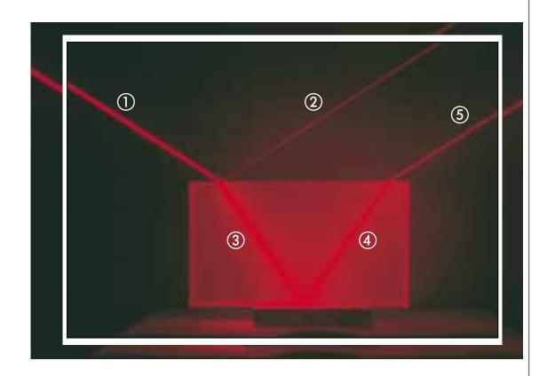
Ray that enters second medium is bent at boundary and is said to be **refracted**Incident ray, reflected ray, and refracted ray all lie in same plane
