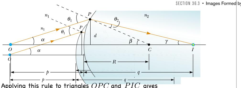
Applying this rule to triangles OPC and PIC gives Figure 36.19 Geometry used to derive Equation 36.8, assuming that  $n_1 < n_2$ .
