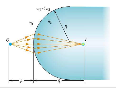
Single ray leaving point  ${\cal O}$  and refracting to point  ${\cal I}$
