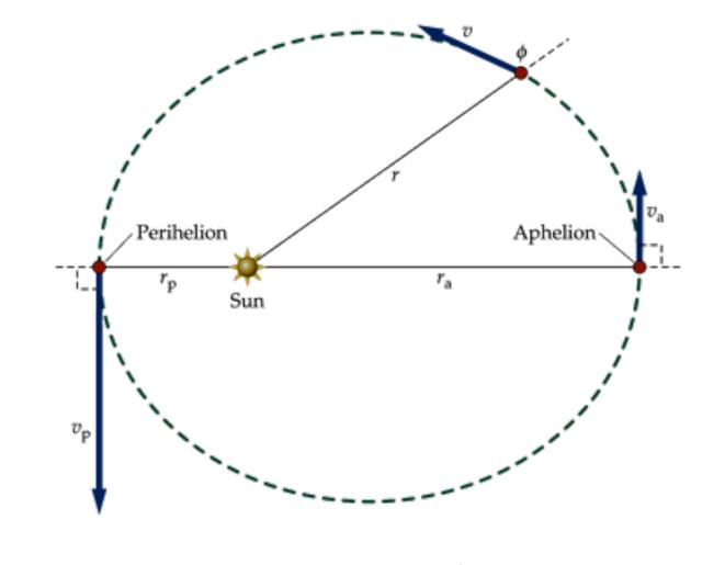
At aphelion and perihelion  $\phi = 90^{\circ} \Rightarrow r_a v_a = r_p v_p$
