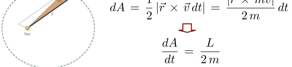
L is angular momentum of planet around Sun Because force of planet is along line from planet to Sun it exerts no torque about Sun L is constant Rate at which area is swept out is same for all parts of orbit
