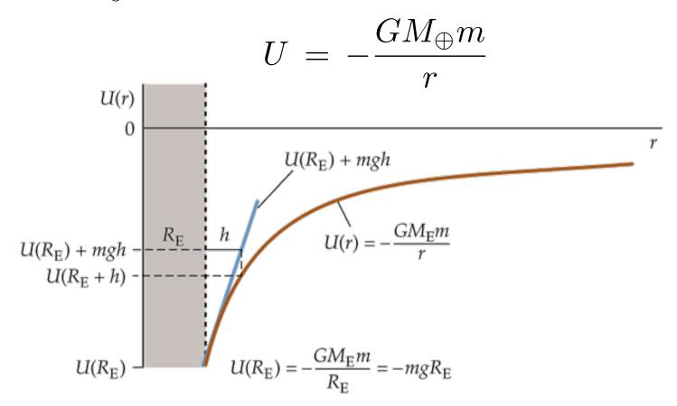
Gravitational potential of Earth starting at surface of planet
