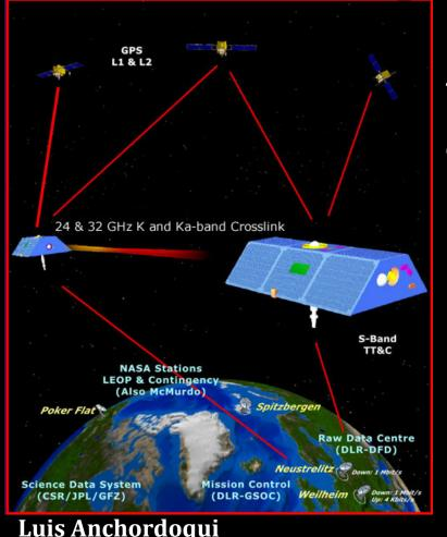
They are in identical orbits with one satellite directly in front of other by about 220 km Distance between satellites is continuously monitored with micrometer accuracy using onboard microwave telemetry equipment How does distance between two satellites <u>changes as satellites approach a region of</u>
