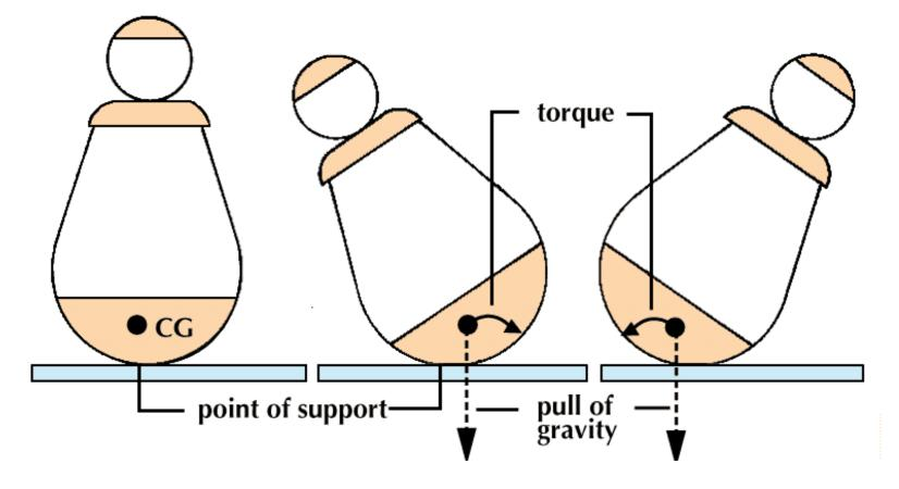
center of gravity average location of the weight of an object
