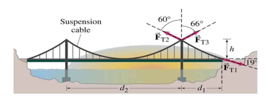
$$\sum F_x = F_{T_1} \cos 19^\circ - F_{T_2} \sin 60^\circ = 0$$
