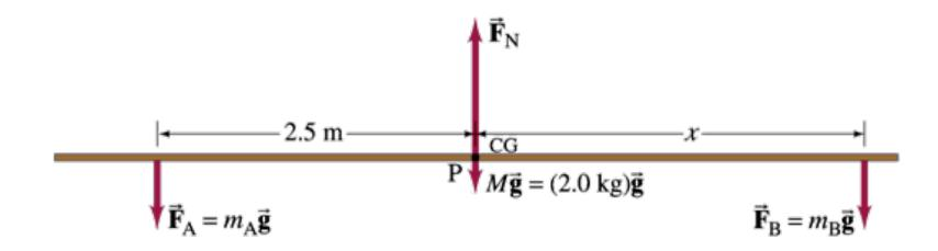
$Mec{g}$  and  $F_N$  make no torque with respect to rotation point
