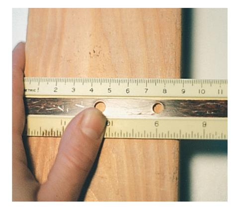
For example, it would be difficult to measure the width of this table to better than a millimeter
