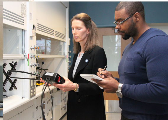
Measuring the rate of airflow into a space is an important step for indoor air quality (IAQ) investigations. —Photos by Phyllis Yip
