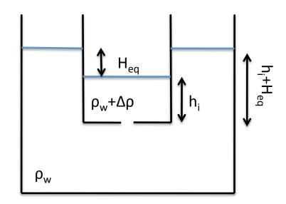
Balance hydrostatic pressures to derive equilibrium height  $(H_{eq})$ :
